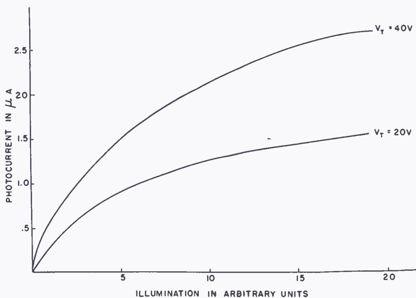
Fig. 3—Photocurrent as a function of illumination for an antimony trisulfide layer with target potential V_T as a parameter.
